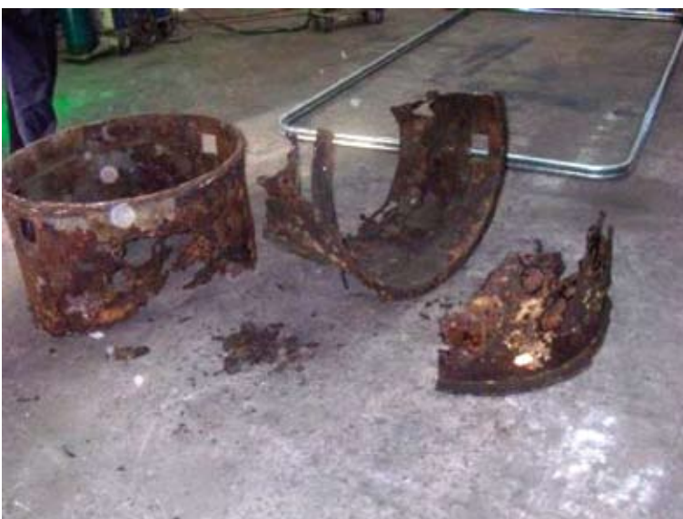
Fire damper casing corroded
