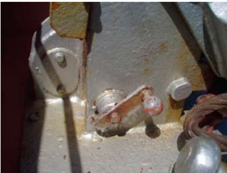
Lifeboat hook locking indicator – horizontal would be locked
