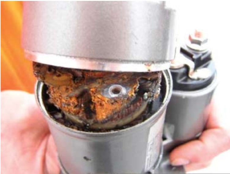
Seized lifeboat engine starting motor internals
